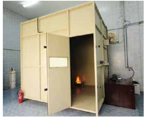
Smoke density 3 m test cube (IEC 61034)
