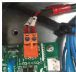
Connection with Outdoor Control PCB Communication Port
