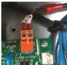
Connection with Outdoor Control PCB Communication Port
