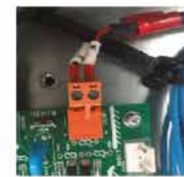
Connection with Outdoor Control PCB Communication Port
